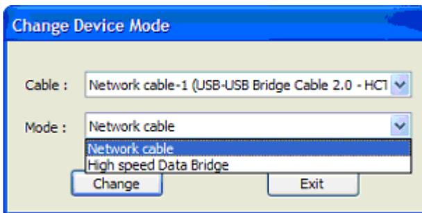
3. If you select Network cable, Windows will detect the Hi-Speed USB-USB Network Adapter and will prompt you automatically to install the software.
