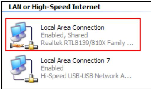
5. Reboot Windows to activate the settings. After Windows has started properly, plug the other end of the USB Bridge-Network cable to the remote computer. Make sure you have run the Setup program on the remote computer as well. Note that you don't need to do the above additional settings for the remote computer.
